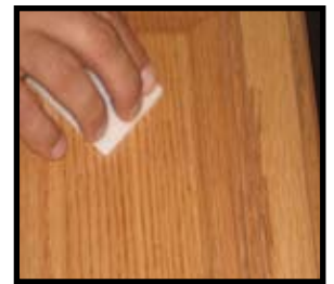
Level with leveling pad
